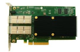
board hardware that off-loads TCP/IP, iSCSI, FCoE and iWARP RDMA processing from its host system. T580-CR frees up host CPU cycles for useful applications. The system achieves increased bandwidth, lower latency, and uses less power.
